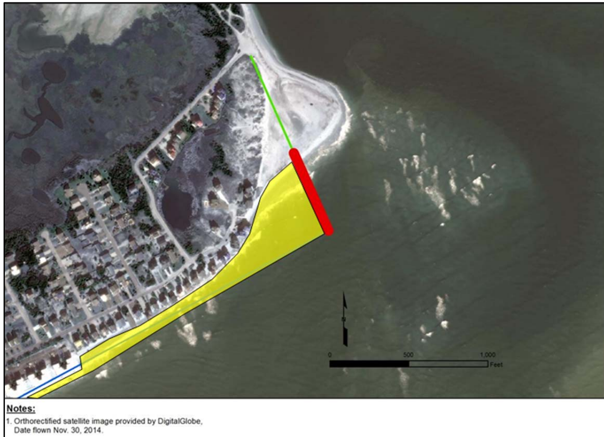
Figure 14. Conceptual rendering of a terminal groin at the north end of North Topsail Beach.
