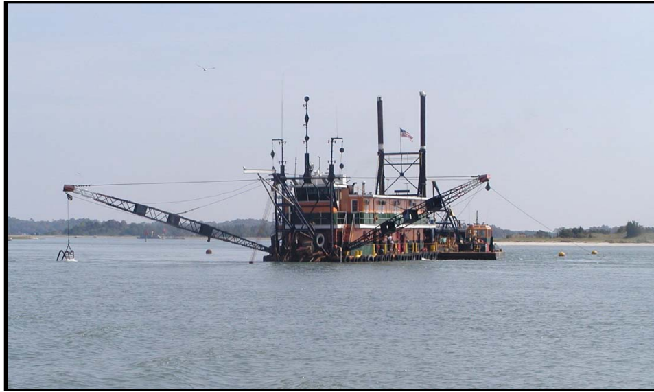
Figure 6. Cutterhead suction dredge comparable to the type used to maintain navigation channels in the AIWW and Channel to Jacksonville (Courtesy Cottrell Contracting Corporation: Dredge Richmond )
