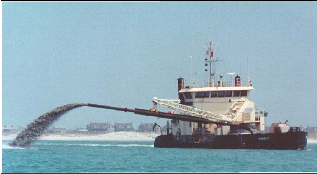
Figure 1. US Sidecast dredge Merritt used to maintain navigation channels in Cedar Bush Cut and the Ocean Bar Channel at New River Inlet (Courtesy of USACE Wilmington District Website).
