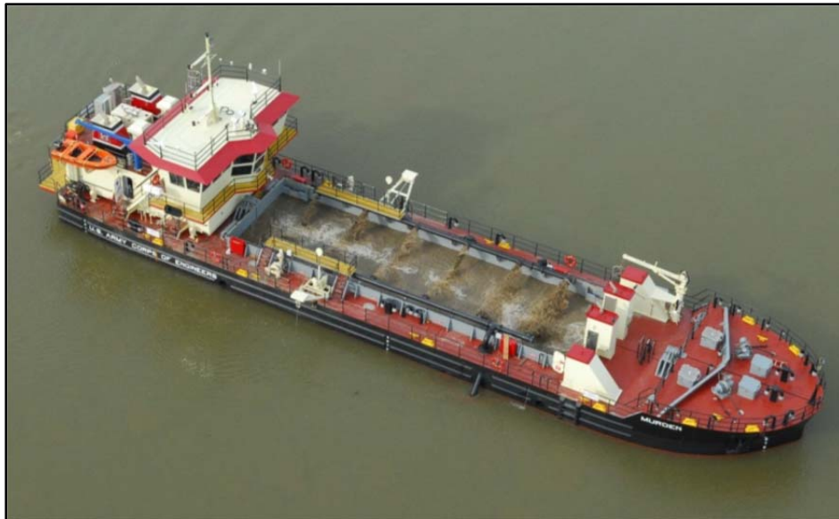
Figure 2. Self-propelled hopper dredge ( Murden ) used to maintain navigation channels in Cedar Bush Cut and the Ocean Bar Channel at New River Inlet (Courtesy of USACE Wilmington District Website).
